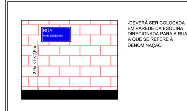
DETALHES DE INSTALAÇÕES DAS PLACAS
